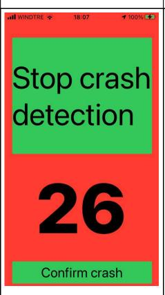
If the crash identification is activated, during the ride if BLEvo identifies the bike on the ground, the crash identification procedure starts and after the timeout, a message will be prepared with the GPS coordinates of the crash and, if selected, the derestriction of the speed is removed.
